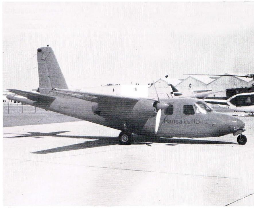
**Aero Commander 680 E equipped for GAMMA-RAY and MAGNETIC FIELD surveys**
