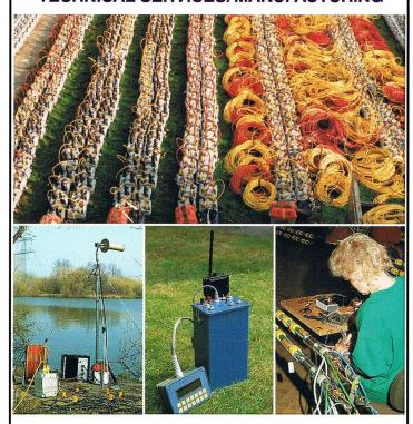
Maintenance of the company's technical outfit is the main task of the division to guarantee the smooth and accurate execution of the company's onshore and offshore operations. In addition to this, electronic tools and geophysical outfit which are not available on the market in the desired quality are tailor-made in the Hannover workshops of the division.
