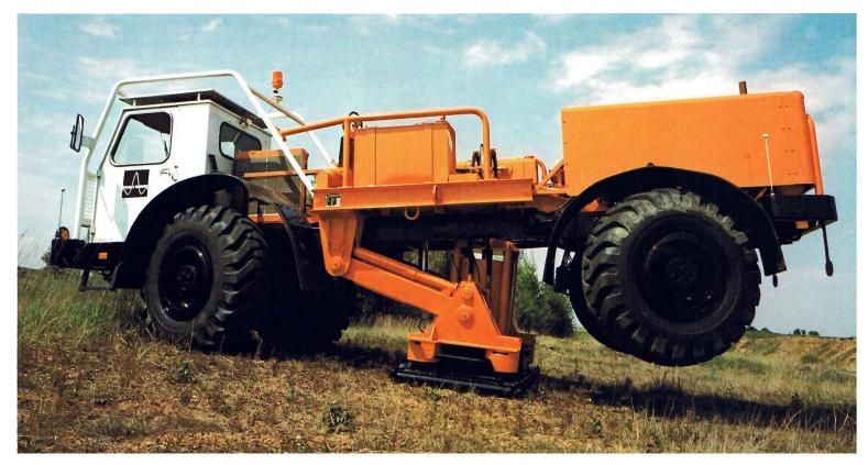
The vibrator type VVCA is an all terrain vibrator approved and equipped for driving and vibrating in european countries but can also be equipped to suit the regulations in other countries with desert areas or
