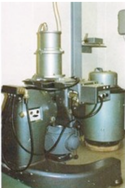
ASKANIA Seegravimeter Gss 3 ASKANIA gravity meter Gss 3 on a survey vessel
