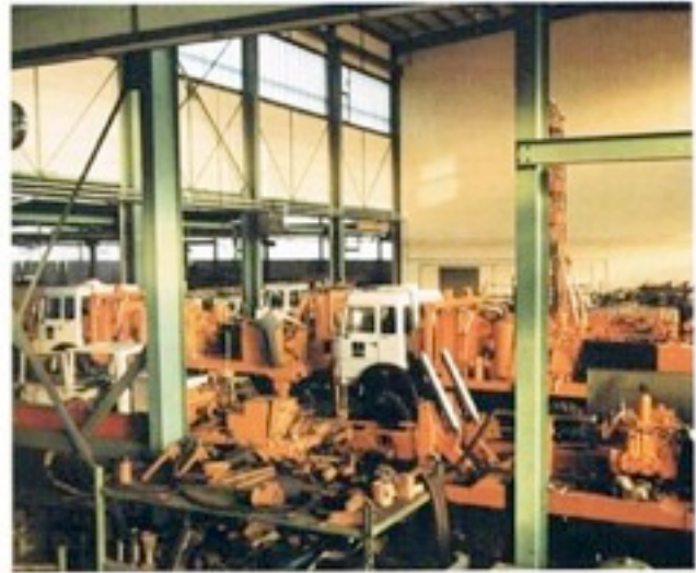
PRAKLA-SEISMOS Geomechanik in Uetze bei Hannover, Bau schwerer Bohrgeräte PRAKLA-SEISMOS Geomechanik in Uetze near Hannover, construction of heavy drilling rigs
