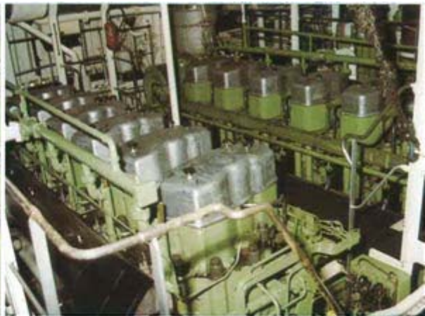
Heart of the ship are the two MaK diesel engines (6 M 551 AK) which drive an Escher-Wyss variable pitch propeller via couplings and reduction gears. The two engines deliver about 4800 HP and produce a ship speed of 15.5 knots.
