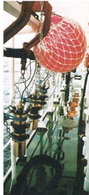
▲ Luftpulserkette Chain with airguns
